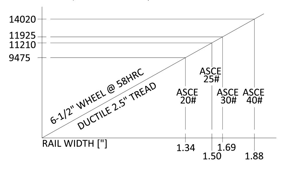
Note: The wheel loads below are not adjusted for duty cycles.
